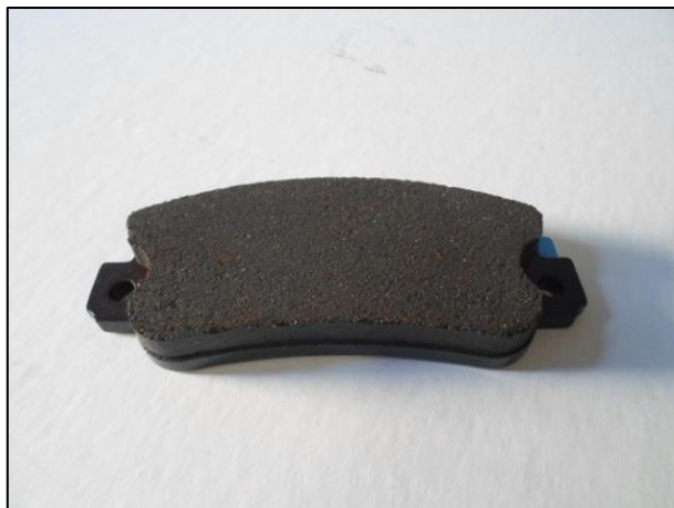
MZHK614 – Pastiglia / Handbrake Pad (OEM 049614)
